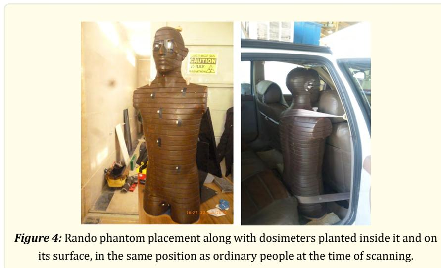
**Figure 4:** Rando phantom placement along with dosimeters planted inside it and on its surface, in the same position as ordinary people at the time of scanning.
