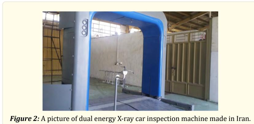
**Figure 2:** A picture of dual energy X-ray car inspection machine made in Iran.
