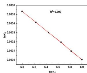
**Figure 3.7:** Van't Hoff plot for methylene blue adsorption onto sawdust.
