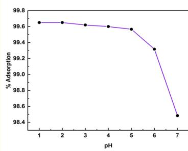
**Figure 1:** Effect of pH on adsorption of Methylene Blue.
