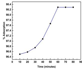
**Figure 2:** Shaking time effect on adsorption of Methylene Blue.
