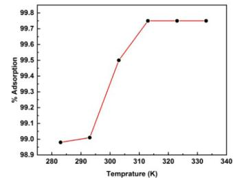
**Figure 7:** Effect of temperature on the adsorption of Methylene Blue.
