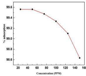
**Figure 5:** Effect of concentration on Methylene Blue removal.
