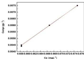
**Figure 6:** Langmuir Isotherm Model for Methylene Blue.
