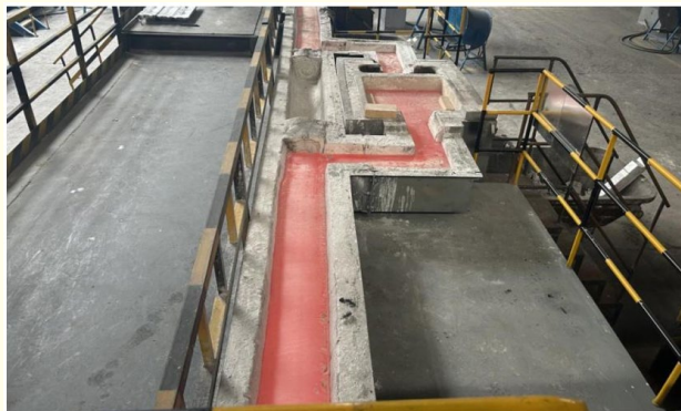
Figure 2: Image of the Plate-Style Filtration Unit in Production.
