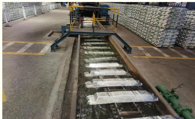
Figure 4: Image of Cooling Process for 3N Aluminum Ingots.
