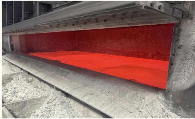
Figure 3: Image of Aluminum Melt After Refining and Slag Removal.
