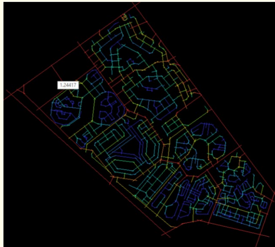
Figure 5: A photo showing integration values of Motamayez district. (Red lines indicate routes with high integration value).
