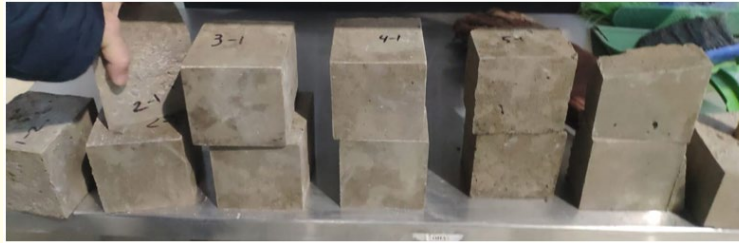
Figure 6: Samples of sulfur concrete for testing.
