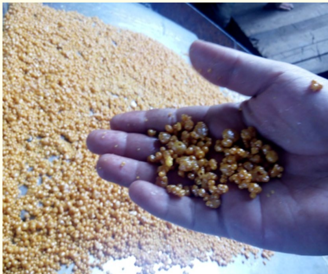
Figure 2: A sample of modified sulfur “Sulfoteks-SB” for the production of sulfur concrete [5].
