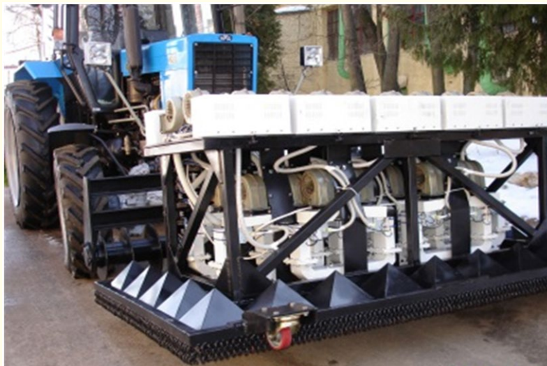
Figure 13: Suspended microwave installation, created by LLC “Center-Novatsiya”, Moscow [3].
