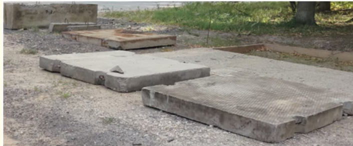
Figure 7: Samples of sulfur concrete for testing.
