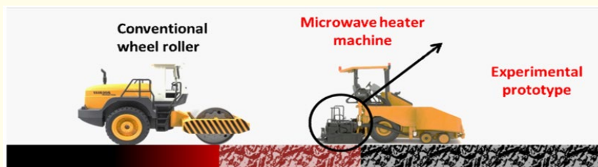
Figure 12: Technology of microwave-induced heating and compacting of the road pavement [3].
