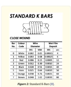
With the required grammage and density of the coating emulsion, the wet film deposit can be calculated, and the correct coating bar can be selected. For example, for the first test with Emulco coating and a desired dry coating grammage of 2 g/m<sup>2</sup>:
