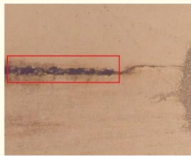
Figure 9: Residual splash between plates.
