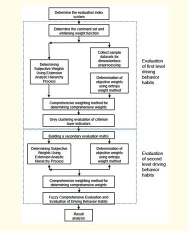
Figure 3: Comprehensive Evaluation Flow Chart of Driving Behavior.
