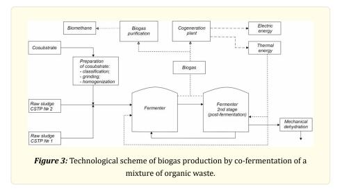
It is proposed to ferment only raw sludge in fermenters, which will allow to increase the specific gas output compared to fermentation of a mixture of raw sludge and excess activated sludge, to refuse the stage of mechanical thickening of excess sludge before fermentation, and to carry out the fermentation process in mesophilic mode, which will significantly reduce costs at this stage of the technological chain.
