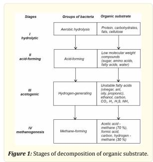
The disintegration of organic substances into components up to conversion into methane can only occur in water environment. Thus, for fermentation of solid substrates it is necessary to add water.
