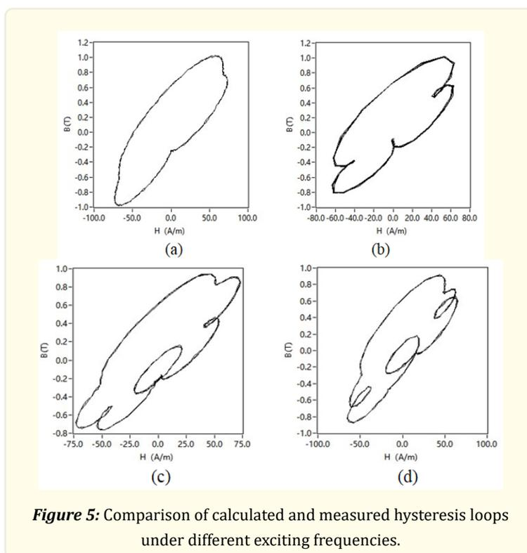
Fig. 5 compares the effect of the controlled harmonic order on the hysteresis loop. (PWM excitation, 8 pulses, modulation index 1.2) When the controlled harmonic order is not more than 3, 5, 7, 9, and the hysteresis loop is as shown in the figure. It can be seen that compared with the sine excitation, the measurement result contains a local hysteresis loop. In addition, the increase of high harmonics will affect the shape and size of the local hysteresis loop.
