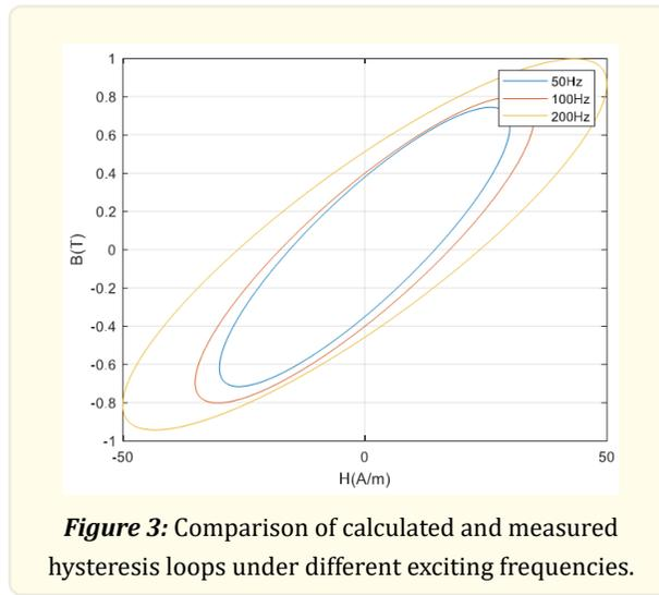
As the excitation frequency increases, the area of the hysteresis loop gradually increases, resulting in an increase in loss.
