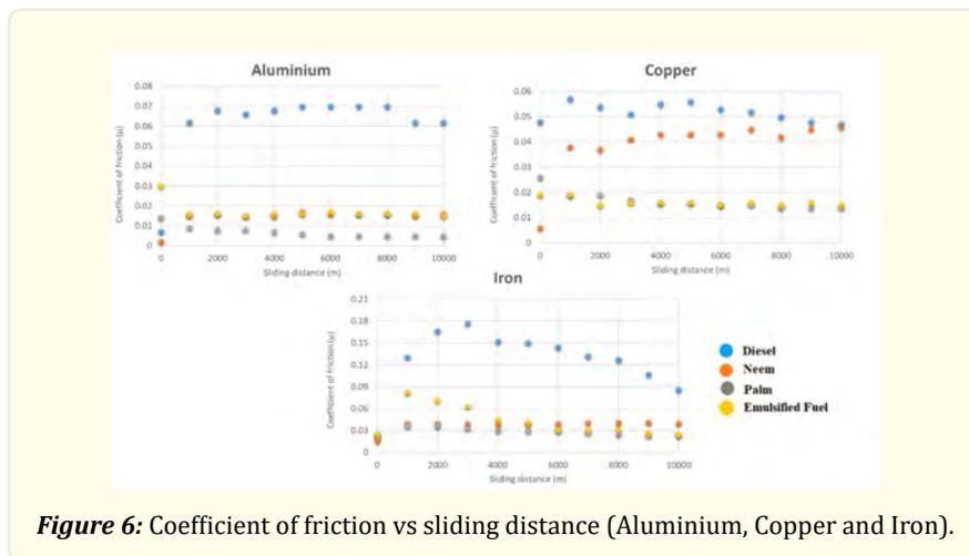
Figure 6: Coefficient of friction vs sliding distance (Aluminium, Copper and Iron).
