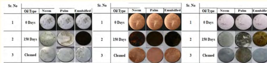
**Figure 3:** Metal coin condition initially, after test and after cleaning corrosion deposits – Aluminium, Copper and Iron.
