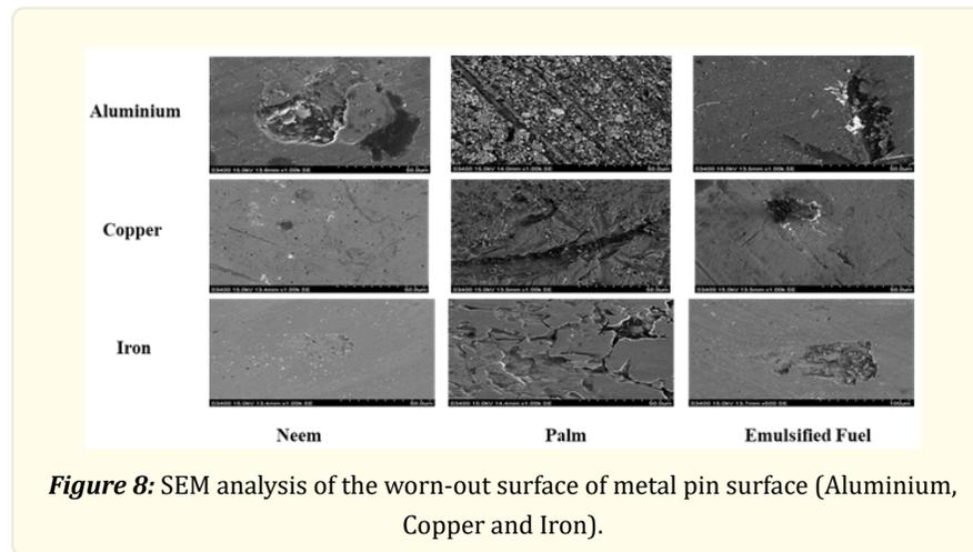
Figure 8: SEM analysis of the worn-out surface of metal pin surface (Aluminium, Copper and Iron).
