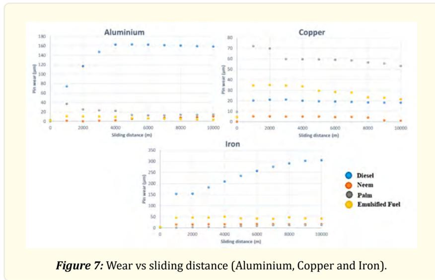
Figure 7: Wear vs sliding distance (Aluminium, Copper and Iron).
