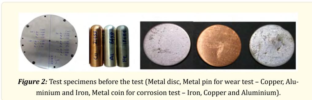
**Figure 2:** Test specimens before the test (Metal disc, Metal pin for wear test – Copper, Aluminium and Iron, Metal coin for corrosion test – Iron, Copper and Aluminium).
