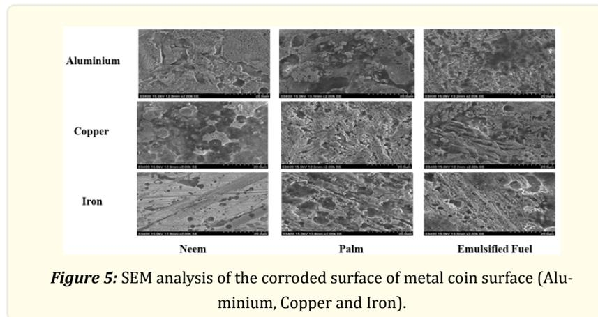
Figure 5: SEM analysis of the corroded surface of metal coin surface (Aluminium, Copper and Iron).
