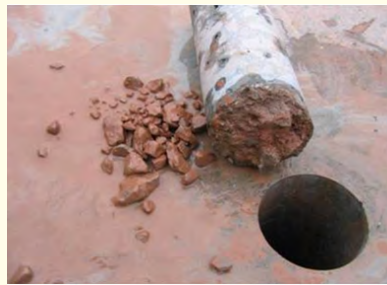
Figure 1: Coring of cement concrete pavement with interlayer coupling between surface layer and base course.
