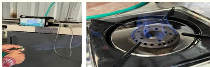
Figure 10: Verification of methane on 2 nd batch.
