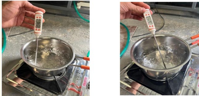
Figure 27: Measurement of temperature required for calorific value of bio gas calculation.
