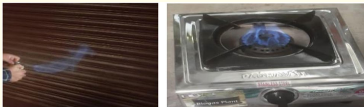
Figure 9: Verification of methane on 1 st batch.
