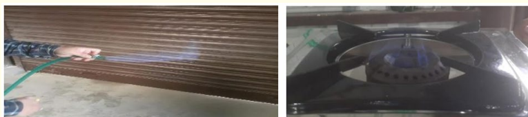
Figure 13: Verification of methane on 5 th batch.
