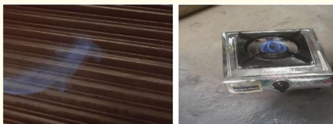
Figure 11: Verification of methane on 3 rd batch.
