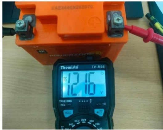
Figure 24: Initial Voltage of Battery.
