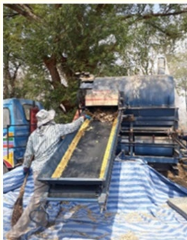
Figure 1: Rice thresher machine Kasetphattana Model tested on Soybean.
