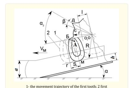
the movement trajectory of the tooth located in the back part of the tooth. *Figure 2:* The scheme for determining the speed of the sprocket teeth of the soil softener-shredder.
