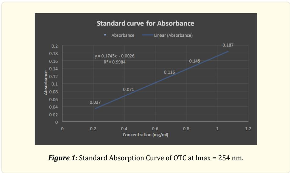
**Figure 1:** Standard Absorption Curve of OTC at  $\lambda_{max} = 254$  nm.
