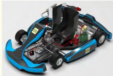
Figure 1: Racing Go-Kart with a single hydraulic disc brake system in rear.
