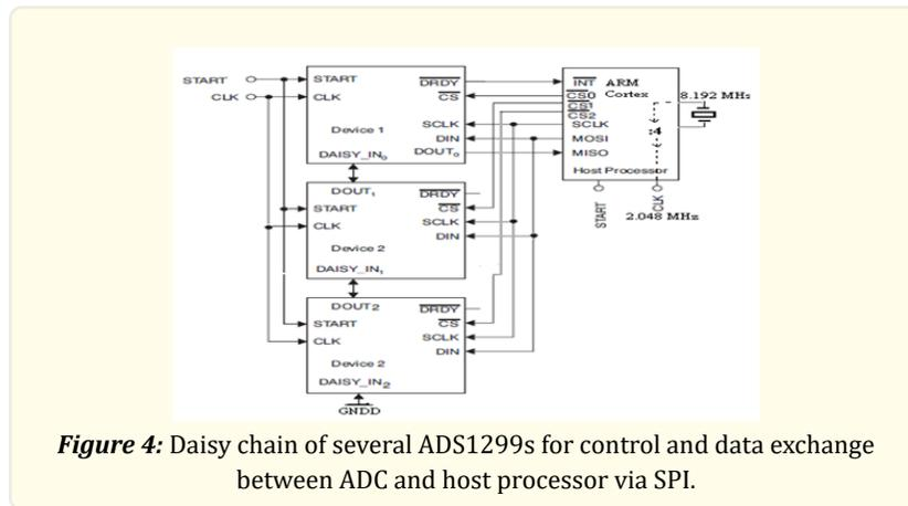
**Figure 4:** Daisy chain of several ADS1299s for control and data exchange between ADC and host processor via SPI.
