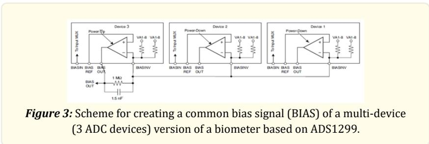
Figure 3: Scheme for creating a common bias signal (BIAS) of a multi-device (3 ADC devices) version of a biometer based on ADS1299.
