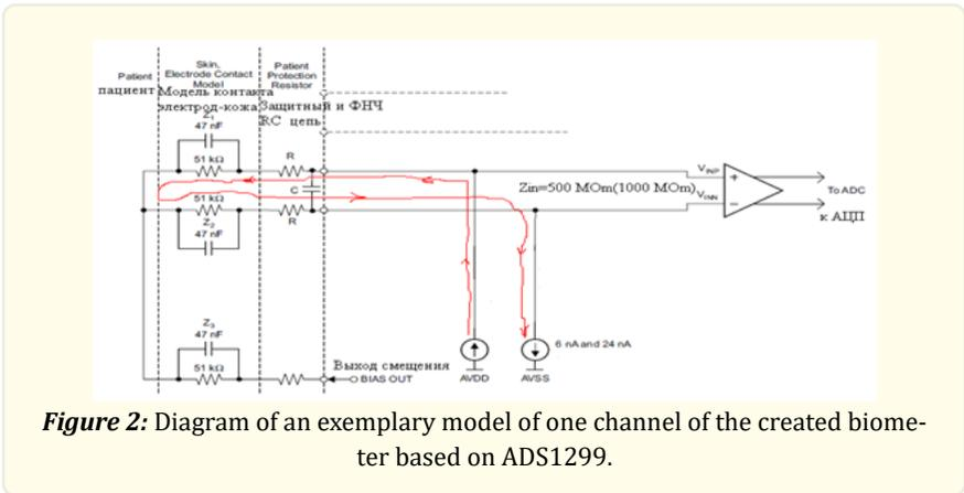
Figure 2: Diagram of an exemplary model of one channel of the created biometer based on ADS1299.
