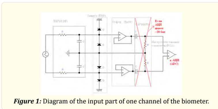
**Figure 1:** Diagram of the input part of one channel of the biometer.
