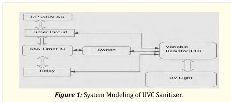
**Figure 1:** System Modeling of UVC Sanitizer.
