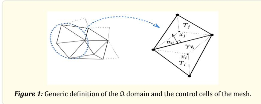
**Figure 1:** Generic definition of the  $\Omega$  domain and the control cells of the mesh.
