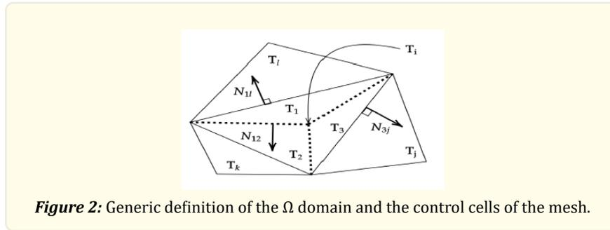
Figure 2: Generic definition of the  $\Omega$  domain and the control cells of the mesh.
