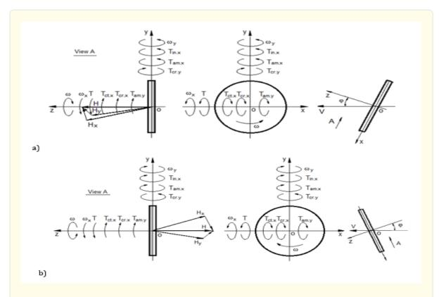
**Figure 1:** The torques and motions acting on the rotating disc in the space station before the first (a) and second (b) inversion.
