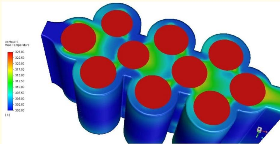
**Figure 15:** Wall temperature distribution contour of Cylindrical-Type Lithium-Ion Battery with Water Liquid Cooling.
