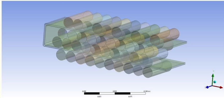
**Figure 9:** 3D model of 40 nos. of Cylindrical Lithium-Ion Batteries with U-Tube Channel Type Water Liquid Cooling system.
