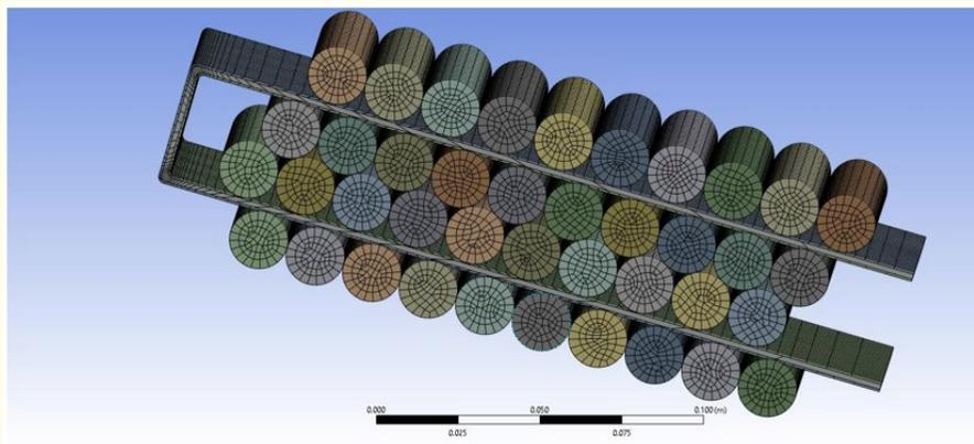
**Figure 10:** Meshing results of 40 nos. of Cylindrical Lithium-Ion Batteries with U-Tube Channel Type Water Liquid Cooling system.
