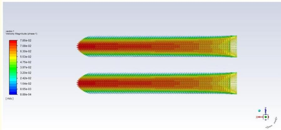
**Figure 14:** Velocity distribution Contour of plate-type lithium-ion battery with Nono fluid coolant channel.
