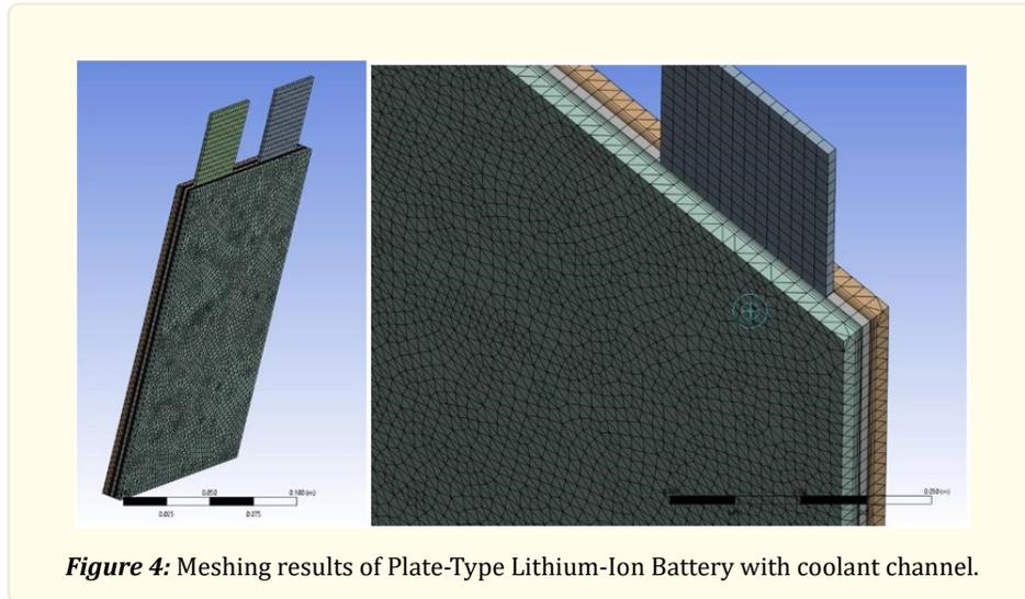
**Figure 4:** Meshing results of Plate-Type Lithium-Ion Battery with coolant channel.
