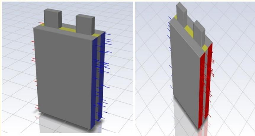
**Figure 5:** 3D model of Plate-Type Lithium-Ion Battery with Nano Fluid Cooling Channel.
