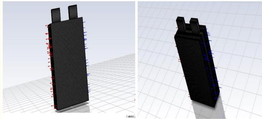
**Figure 6:** Meshing results of Plate-Type Lithium-Ion Battery with Nano Fluid Cooling Channel.
