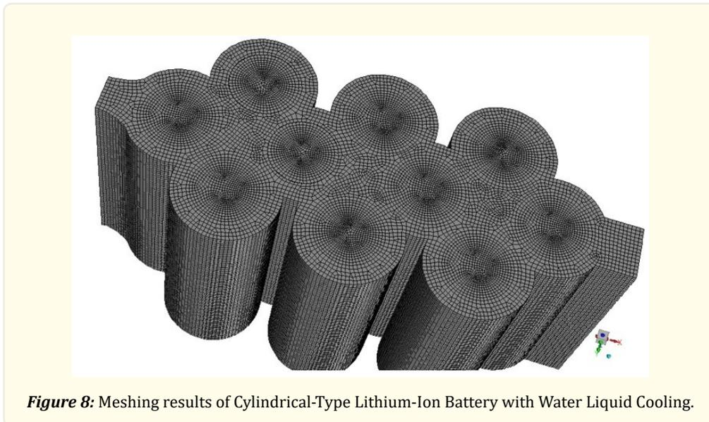
**Figure 8:** Meshing results of Cylindrical-Type Lithium-Ion Battery with Water Liquid Cooling.
