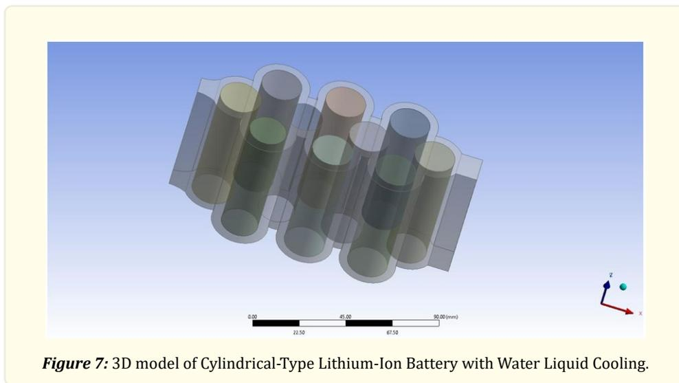
**Figure 7:** 3D model of Cylindrical-Type Lithium-Ion Battery with Water Liquid Cooling.
