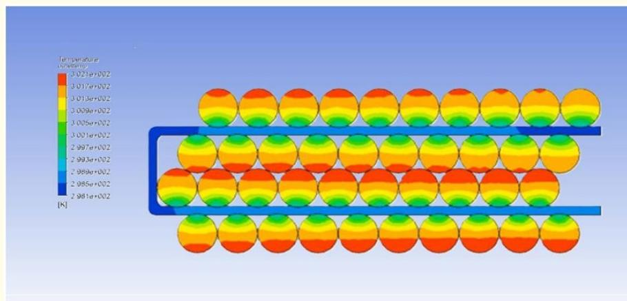
**Figure 16:** Temperature distribution contours of 40 nos. of Cylindrical Lithium-Ion Batteries with U-Tube Channel Type Water Liquid Cooling system.
