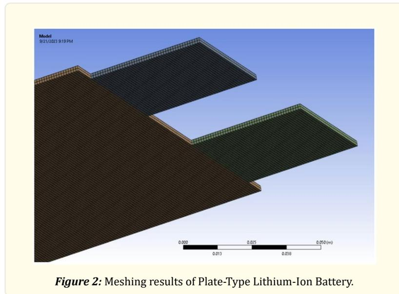
**Figure 2:** Meshing results of Plate-Type Lithium-Ion Battery.
