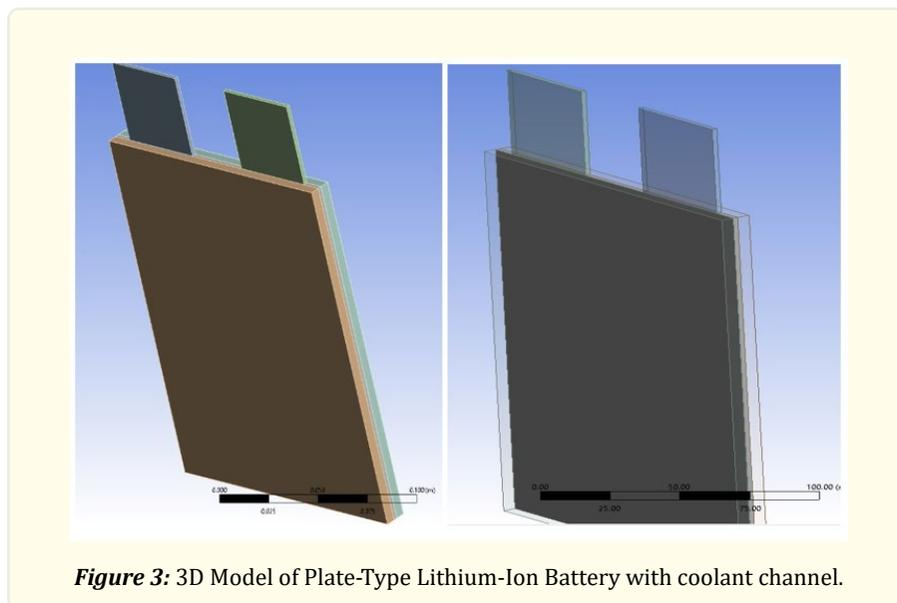
**Figure 3:** 3D Model of Plate-Type Lithium-Ion Battery with coolant channel.
