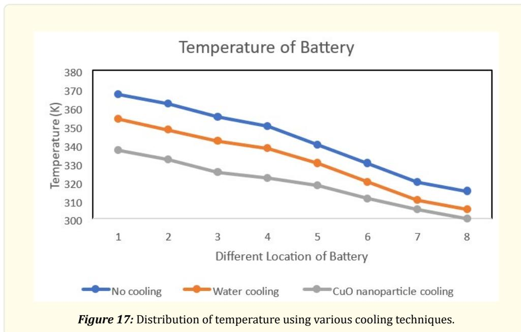
**Figure 17:** Distribution of temperature using various cooling techniques.
