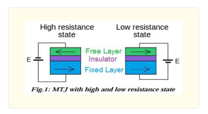
Here we have exploited the above-mentioned properties to realize the universal NAND and NOR logic gates [7] with a simple behavioral model of MTJ device (shown in Fig. 2) which has been represented as two identical diodes with a low resistance (RP) during parallel magnetization and high resistance (RAP) during anti-parallel magnetization.
