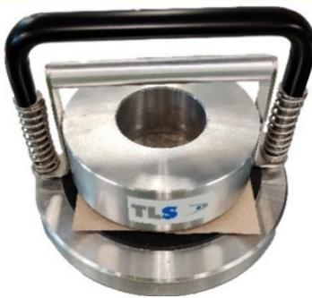
**Figure 3:** Cobb test cylinder.
