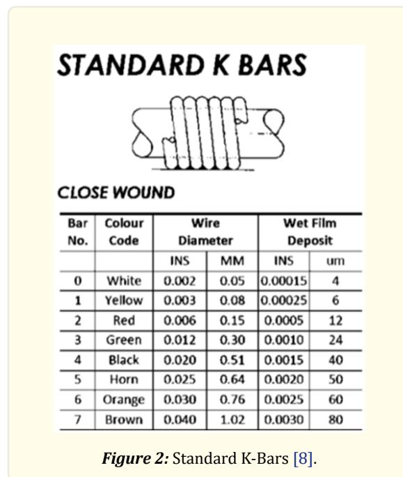
With the required grammage and density of the coating emulsion, the wet film deposit can be calculated, and the correct coating bar can be selected. For example, for the first test with Emulco coating and a desired dry coating grammage of 2 g/m<sup>2</sup>:
