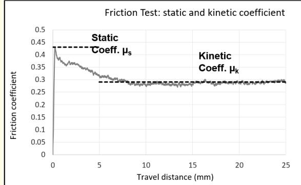
**Figure 7:** Friction test: static and kinetic coefficient.
