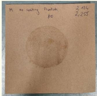
**Figure 4:** Cobb test sample.
