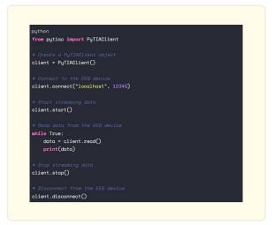
This code creates a PyTIAClient object and connects to an EEG device running on the local machine at port 12345. It then starts streaming data from the device and reads the data in a loop. Finally, it stops streaming data and disconnects from the device.
