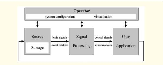
Figure 1: A schematic block diagram of the BCI2000 system. BCI2000 design. BCI2000 consists of four modules: operator, source, signal processing, and application. Operator module acts as a central relay for system configuration and online presentation of results to the investigator. It also defines onset and offset of operation. During operation, information (i.e., signals, parameters, or event markers) is communicated from source to signal processing, to user application, and back to source.
