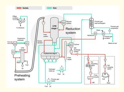
Figure 1: A simplified process flow diagram of the Circored process.
