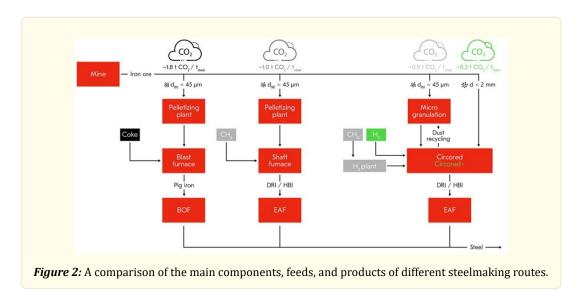
It is apparent that the BF/BOF route is by far the largest emitter of  $CO_2$ ; furthermore, the technical solutions to minimize emissions are limited for this route. While the  $CO_2$  emissions of the Circored process and shaft furnace direct reduction are in the same order of magnitude, Circored benefits from the omission of the pelletizing step. As the Circored+ process is designed to produce fully green steel, its  $CO_2$  emissions are negligible.
