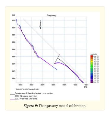
The calibrated model is used for the prediction of shoreline oscillations around the breakwaters constructed for the harbour at Thangassery. The shoreline evolution results are predicted after  $5^{th}$ ,  $10^{th}$  and  $15^{th}$  years. The final result is presented in Fig. 10.
