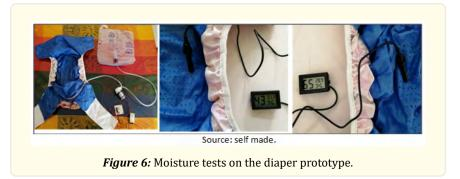
The maximum humidity found is 70%. It takes approximately 10 to 20 minutes to lower the humidity from the maximum limit to the initial limit. But it takes about 8 minutes to go down from the maximum limit to a medium limit.
