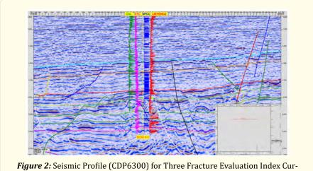
**Figure 2:** Seismic Profile (CDP6300) for Three Fracture Evaluation Index Curves(RTC SPCC LIEFENG2) of #5 Well.
