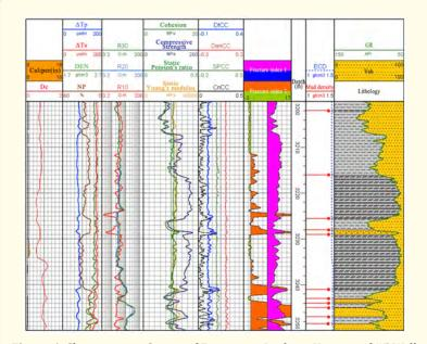
Figure 1: Characteristic Curves of Fracture at Leakage Horizon of #5 Well.
