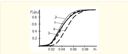
*Figure 4:* Dependences of probability of error in RS-codes on probability of bit error. 1 - m = 5, t = 5; 2 - m = 6, t = 5; 3 - m = 6, t = 7; 3 - m = 6, t = 10.
