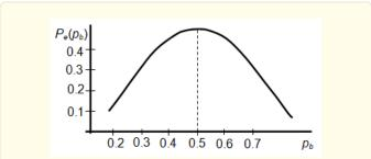
**Figure 5:** Dependence of the probability of error in convolutional code on probability of bit error.
